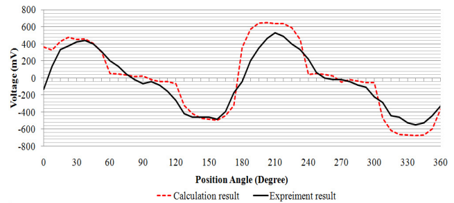
Fig. 3. Comparison of V_{BC} variation between the experiment result and simulation results.
